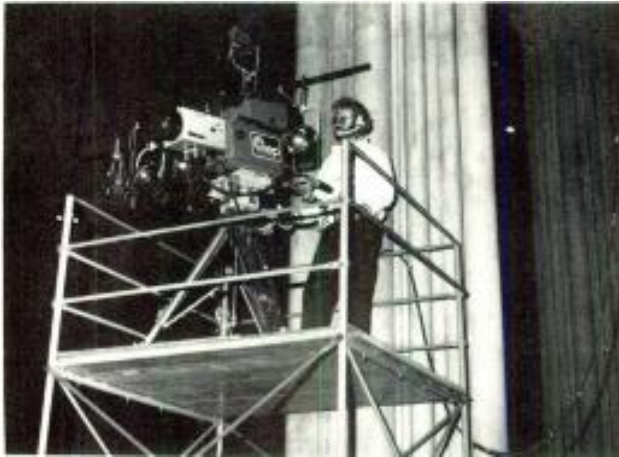
Using Hitachi SK 96s with 22:1 Fujinon zoom lenses, supplied by NEP, WPIX-TV, NY, provided free public service broadcast of St. Patrick's Christmas Eve Mass to 33 INN affiliates. CSI lights were used to provide 250 fc illumination to selected areas of the gloomy interior.
