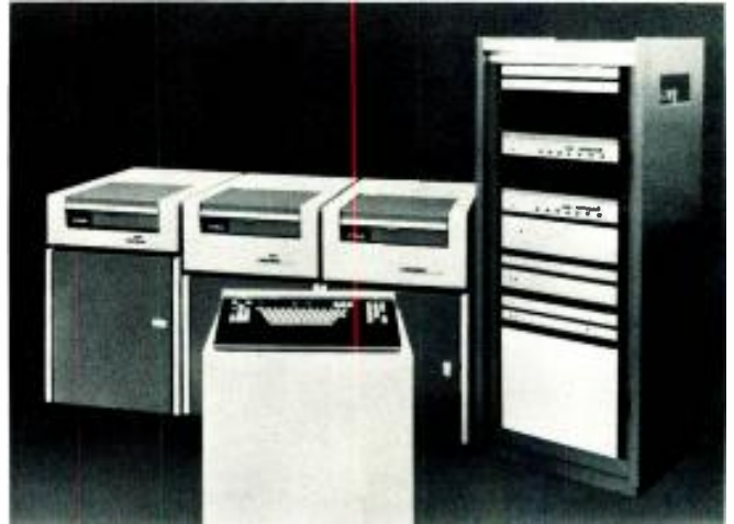
The Harris IRIS still store can accommodate up to eight disk drives with a total system capacity of 740,000 stills.
