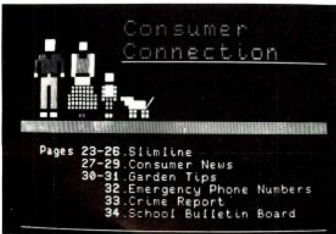
Teletext graphics are extremely low resolution, dependent on the alphanumeric character base.
